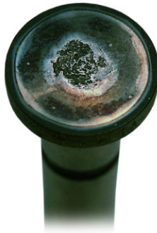
Lycoming follower after 240 hours with Competitive Semi-Synthetic 15W-50 Multi-grade.
