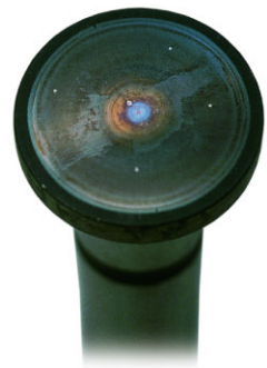
Lycoming follower with virtually no pitting after 300 hours with Exxon Elite 20W-50.
