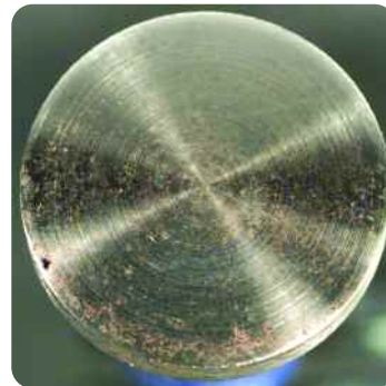
Commercial AD Monograde claiming to meet the Lycoming antiwear-antiscuff additive requirement (SAE 50)
