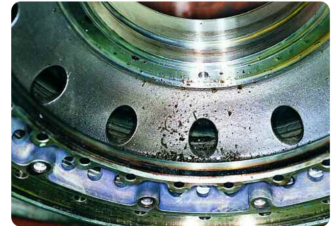
CFM56-3C1 Number 5 Bearing — Rear Compartment Mobil Jet Oil II: 20,600 hours, 7,300 cycles Minimal deposits with Mobil Jet Oil II.
