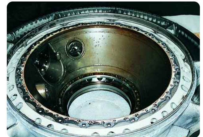
RB.211-535C 03 Module — Walls with Gears Removed Mobil Jet Oil II: 18,500 hours, 13,400 cycles Sump walls are clean and free from deposits with only a slight brown discoloration.
