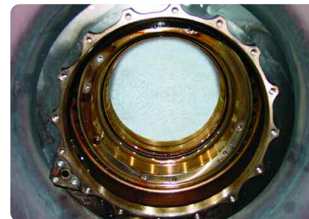
PW2040 Number 5 Bearing/Seal Housing Mobil Jet Oil II: 17,336 hours, 10,708 cycles Excellent condition with light varnish deposits.
