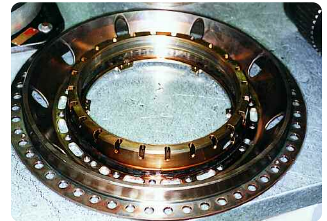
CF6-80C2B1F Number 5 Bearing Housing Mobil Jet Oil II: 13,700 hours, 2,200 cycles Minimal deposits with Mobil Jet Oil II.
